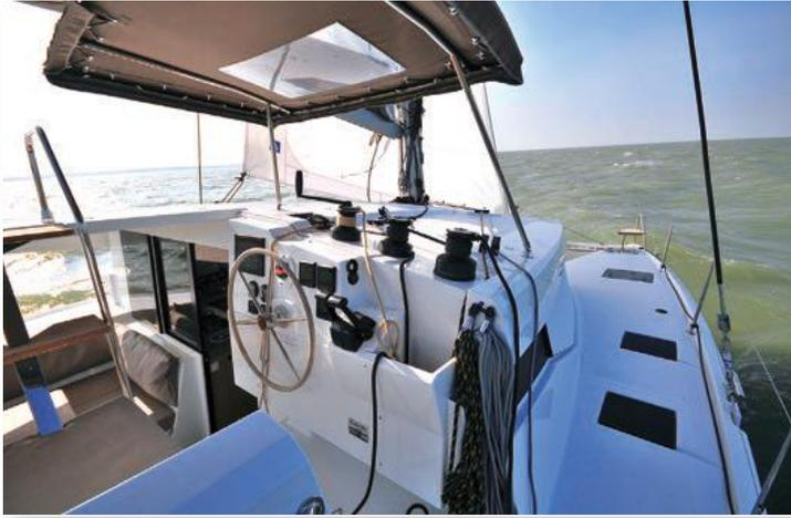
↑ All sail-handling is led back to the helm station, not too exposed, preserving the overall lines. Note the stowage box for lines and the straps for the coiled halyards
