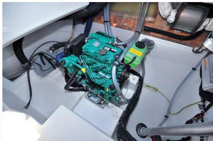
→ An engine compartment with room to work. Note the compact balsa/glass sandwich. A hatch shuts off the aft of the compartment where there is polystyrene for buoyancy, though I would have preferred to see a dense foam.
